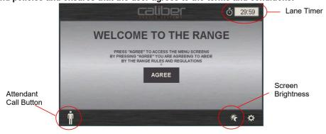
The lane control screen also contains an "Assistance" acceptance button which engages a call light on the drive unit to visually alert the range operator that assistance is required. This allows the shooter to maintain their position in the lane while waiting for assistance, minimizing movement behind the firing line and enhancing range safety. In addition, the lane control will display any fault or alarms to alert the user of an issue with the system.
