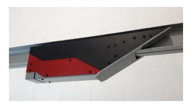
The target carrier travels along a rugged steel "I" beam track and its position is tracked using an encoder, which gives reliable and repeatable positioning to within ± 1 inch (2.5cm). The front of the carrier is protected by a 1/4" AR steel angled plate that deflects errant rounds safely while also protecting internal components.
