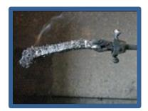
EXP® Rubber self-extinguishes during UL 94 test
