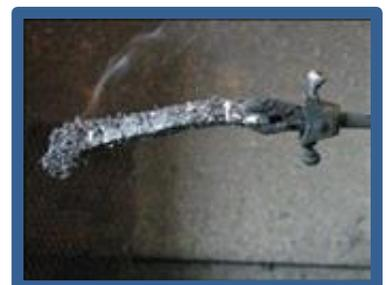
EXP® Rubber self-extinguishes during UL 94 test
